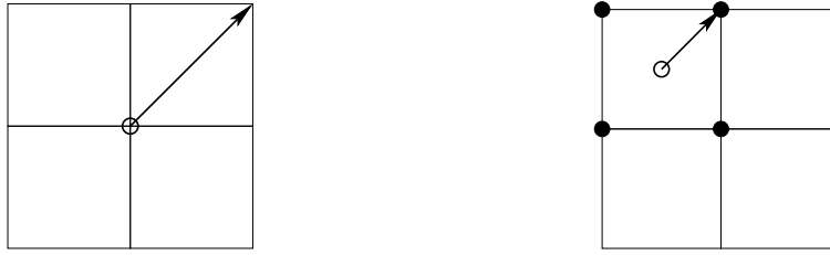
Figure 3.2: Example of the quality computation of a 2 \times 2 square. Ideal case on the left, discrete case on the right. Note that the centers are different (circles). In the discrete case the coordinates of each tile is also shown (solid dots). The maximum radius is marked with an arrow. The quality in the ideal case is Q_{ideal} = \frac{4}{(\sqrt{2})^2} = 2 < \pi . The discrete case however has a quality of Q_{discrete} = \frac{4}{(\sqrt{2}/2)^2} = 8 > \pi .
